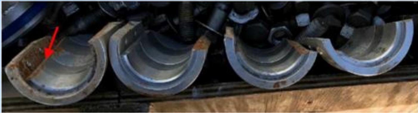
Broken shaft coupling sleeves, typical break patterns
